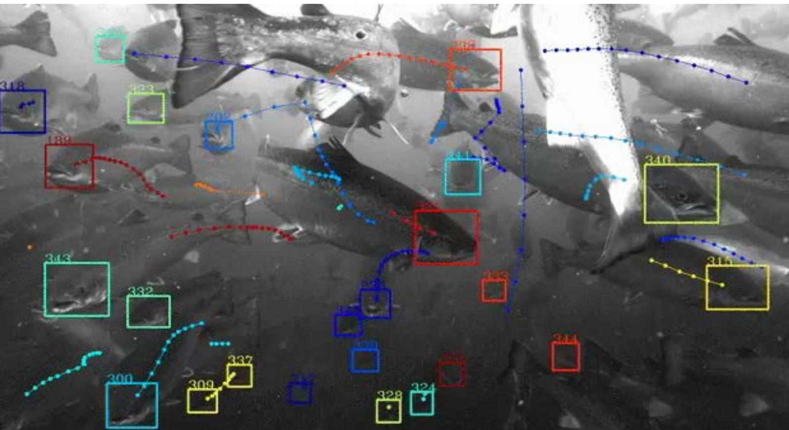
Picture: Tidal's underwater system interpreting feeding behavior by tracking objects in the water
