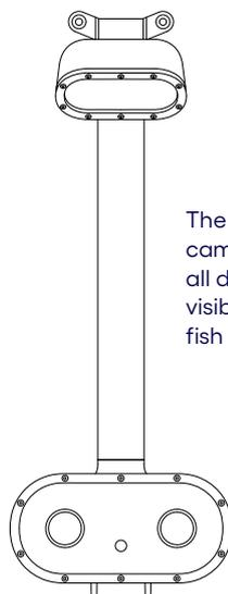
The "Hammerhead" camera adjusts in all directions for full visibility inside the fish pen.
